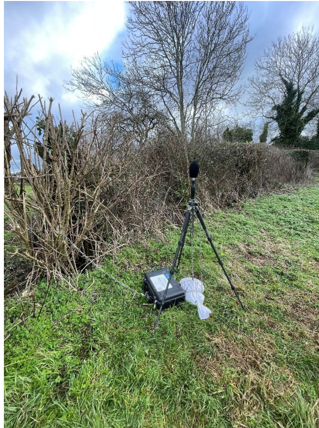
Figure 10-2 Unattended Noise Measurement Setup
