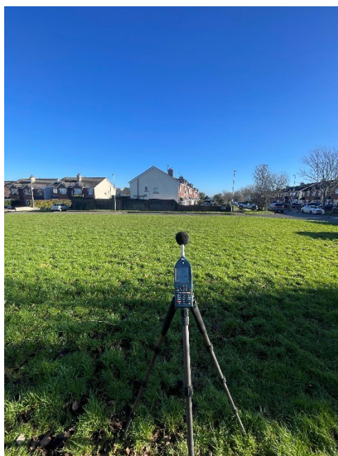
Figure 10-3: Attended noise measurement setup.
